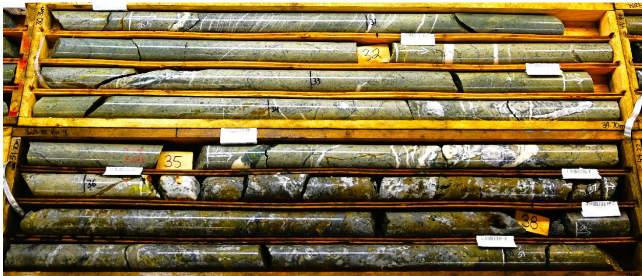
Figure 3: Massive replacement-style pyrite, sphalerite, chalcopyrite in contact with dioritic intrusive analog to the Goldslide intrusive at the Willow Zone in hole W21-115 grading 4.95 g/t AuEq over 9.88 m.
