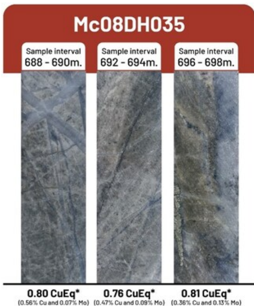
Figure 3 – Deep porphyry mineralization observed at the end of the hole Mc08DH-035 (total depth of 699.13m) drilled by B2gold in 2008. Note the historical CuEq* grade for each sample length. Left: Kspar altered dacite porphyry with stockwork of B-type veins (moly and minor chalcopyrite). Center: Kspar altered dacite porphyry with overprinted sericite, with A-type veinlets cross-cutting by B-type veinlets (only moly type). Right: Kspar altered dacite porphyry with overprinted sericite, with B-type veinlet (quartz + moly) cross-cutting by late D-type vein (pyrite + minor quartz content). (CNW Group/Libero Copper & Gold Corporation)
