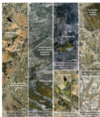
Figure 2 - MD-045 - Brecciation stage at the Moco porphyry system. *Moly (molybdenite) (CNW Group/Libero Copper & Gold Corporation)
