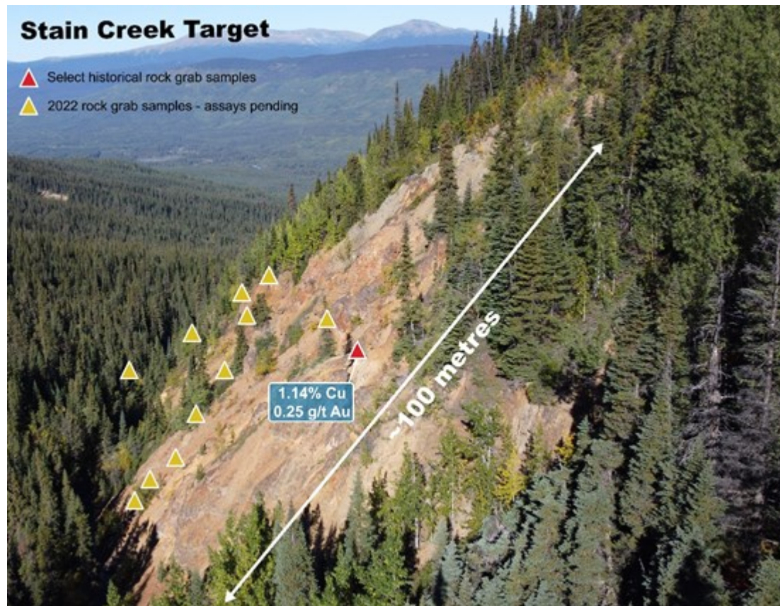
Figure 3. Highly altered gossanous outcrop exposure largely composed of a syenitic intrusion, with select historical rock grab sample locations with the Stain Creek target area. Further sampling of the section was conducted during Torr's 2022 exploration program.
