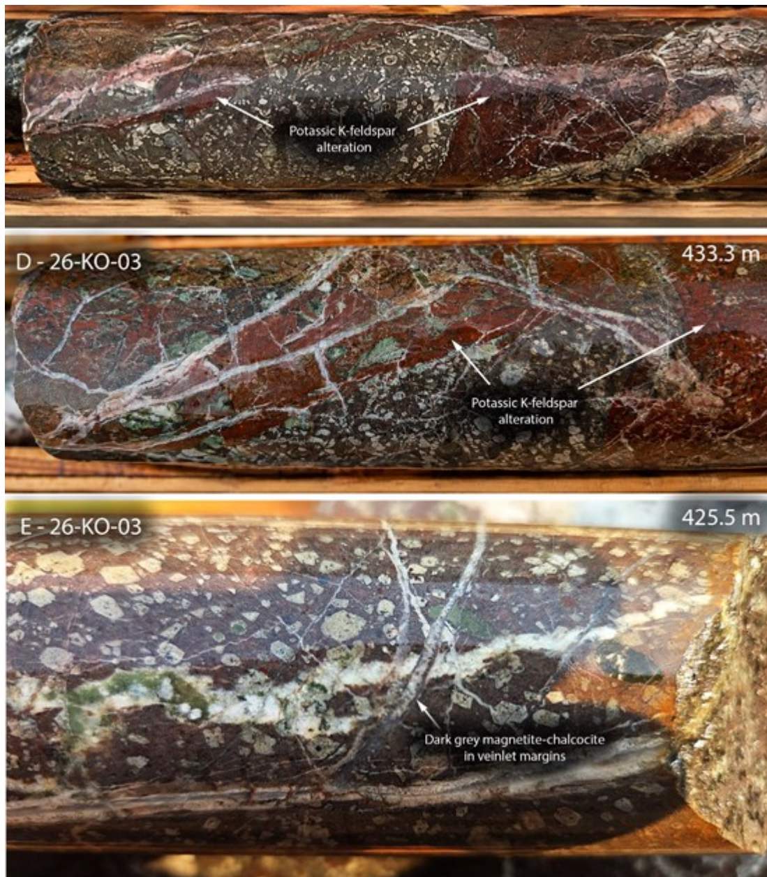
Figure 1. Representative red (hematized) drill core showing pyrite-chalcopyrite and native copper mineralization in drill hole 26-KO-04 (A-B), intrusive rocks affected by intense reddish interpreted K-feldspar alteration (B-C), hydrothermal brecciation and multiple generations of cross-cutting veinlets and stockwork within a broader overprinting sericitic alteration corridor (D). Dark grey material (D) interpreted as magnetite with chalcocite occurring in veinlet margins. Alteration and mineral identification remain subject to petrographic, geochemical and laboratory confirmation.
