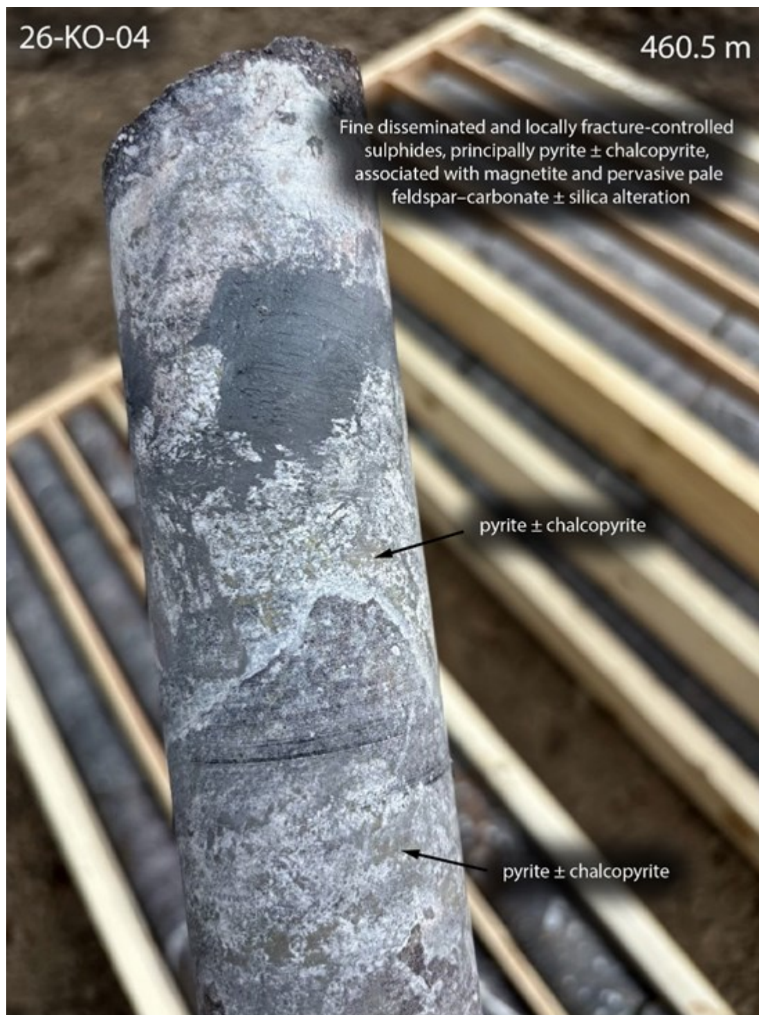
Figure 1. Hole 26-KO-04 at approximately 460.5 m showing a select magnetite-bearing intrusive dyke with disseminated pyrite-chalcopyrite mineralization within a broader brecciated volcanic and mineralized interval from approximately 429.2 to 469.8 m. Mineral and alteration identifications remain subject to petrographic, geochemical and laboratory confirmation.
