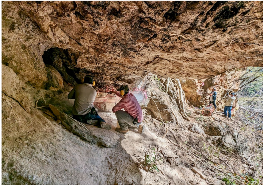
Figure 3 Cutting a channel sample in large outcrop at El Cometa.
